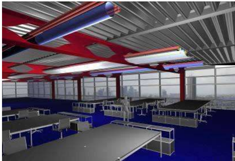
Integration of all the services in the height of the beam using Angelina™
